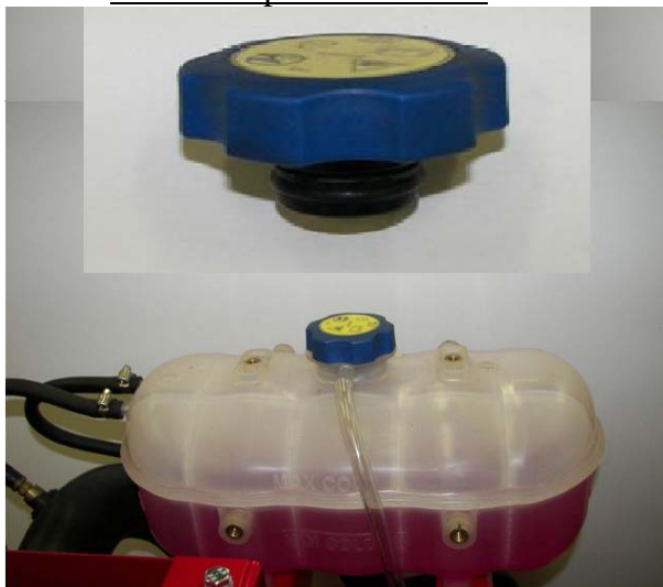
Photo of Existing Pressure Cap/Tank
