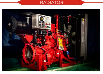
Radiator cooled engines have coolant that is sent to the radiator. The coolant flows through tubes that penetrate through the fins. An engine driven fan blows air across the radiator fins, which then removes the heat from the coolant. The coolant then travels back to the engine block through the engine water pump and the cycle continues while the engine is running.
